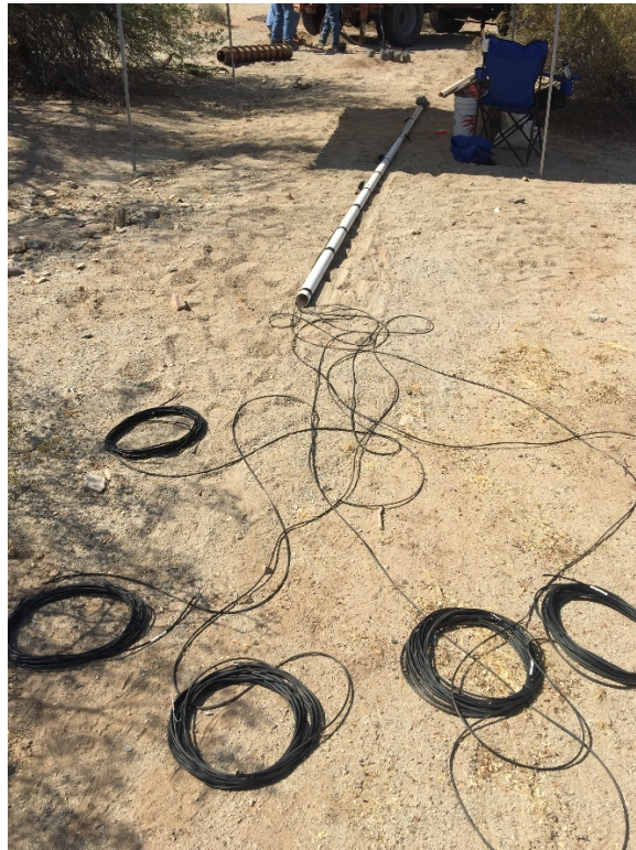
July 7, 2017 HSP-2 well casing with soil moisture sensor cables before installation in the drill borehole.
