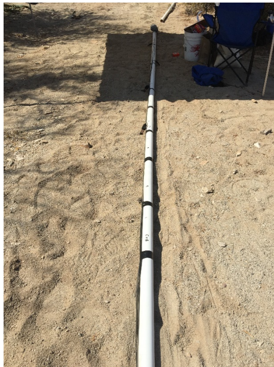
July 7, 2017 HSP-2 well casing with soil moisture sensors attached to casing before installation in the drill borehole.
