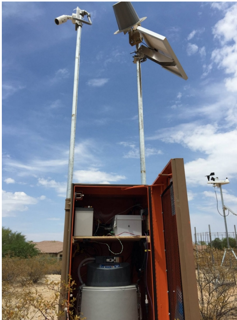
6/27/17 USGS install surface water monitoring station at HSP study area.
