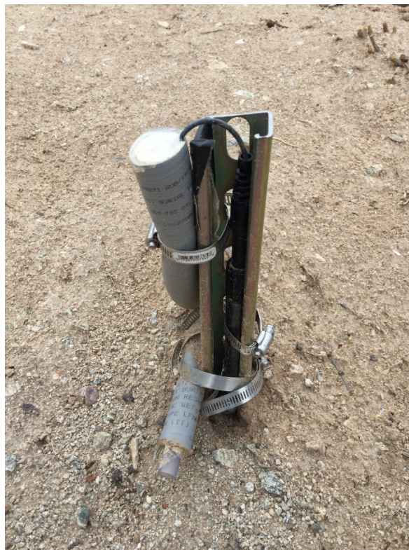
USGS main surface water sensor connected to water monitoring station.
