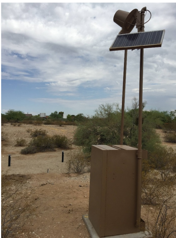
7/21/17 USGS surface water datalogger housing, a USGS surface water sensor at the edge of the channel, and groundwater wells HSP-1 and HSP-2. Photo looking north.
