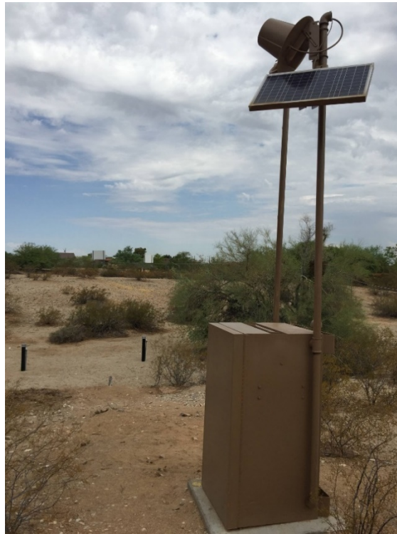
USGS surface water datalogger housing, a USGS surface water sensor at the edge of the channel, and groundwater wells HSP-1 and HSP-2. Photo looking north.
