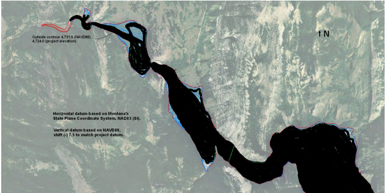
Figure 8 - Gibson Reservoir, multibeam bathymetric data in upstream area (NAVD88).
