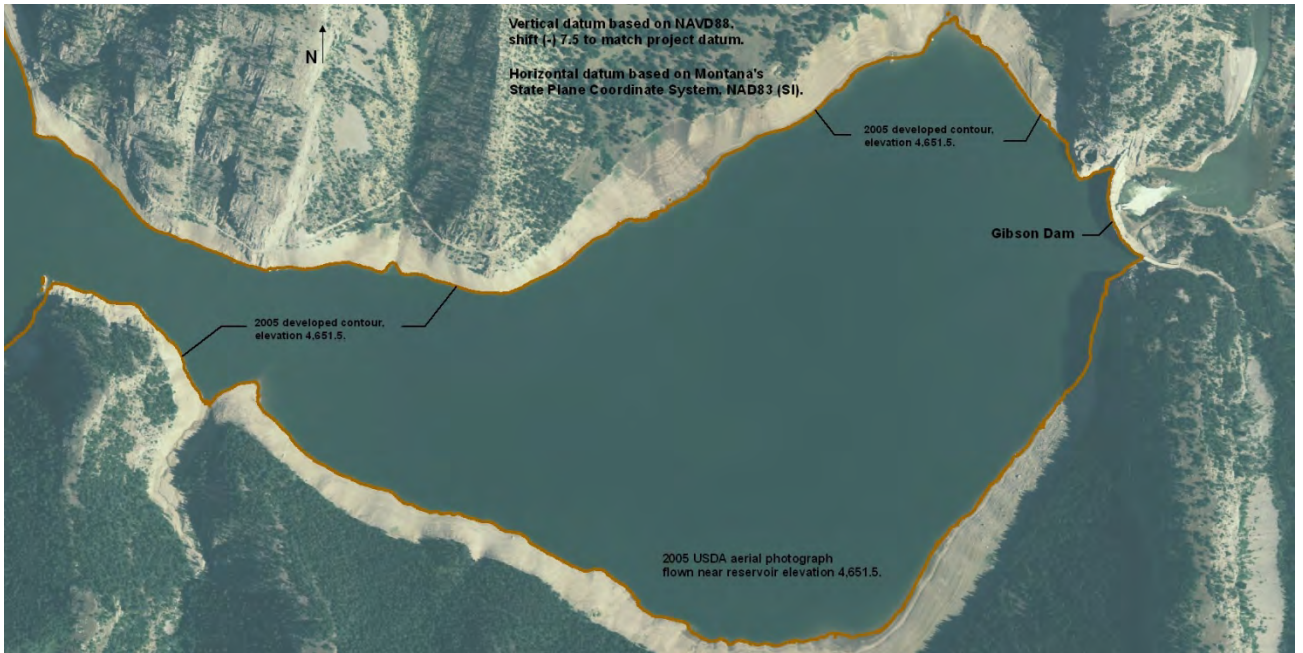
Figure 10 - Aerial image of Gibson Dam and Reservoir at water surface elevation 4,651.5 (NAVD88), flown in 2005 (USDA, 2010).
