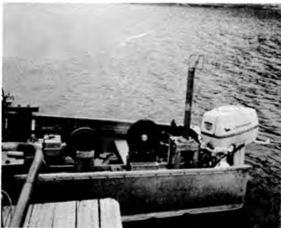
Figure 8. Distance measuring machine mounted in back of the boat. Fair lead for piano wire guidance can be seen at right. It has a periscope appearance. Photo P258-D-57703
