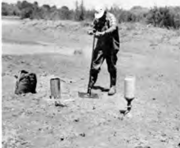
Figure 12. Taking a sediment sample with field density apparatus. Photo P258-D-57697
