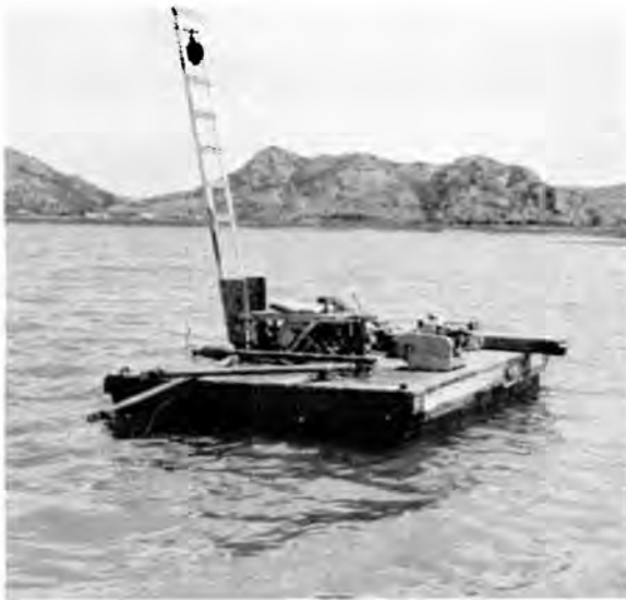
Figure 10. Gravity core sampler shown suspended from a cable and lying on the platform of the raft. Photo P258-D-57699
