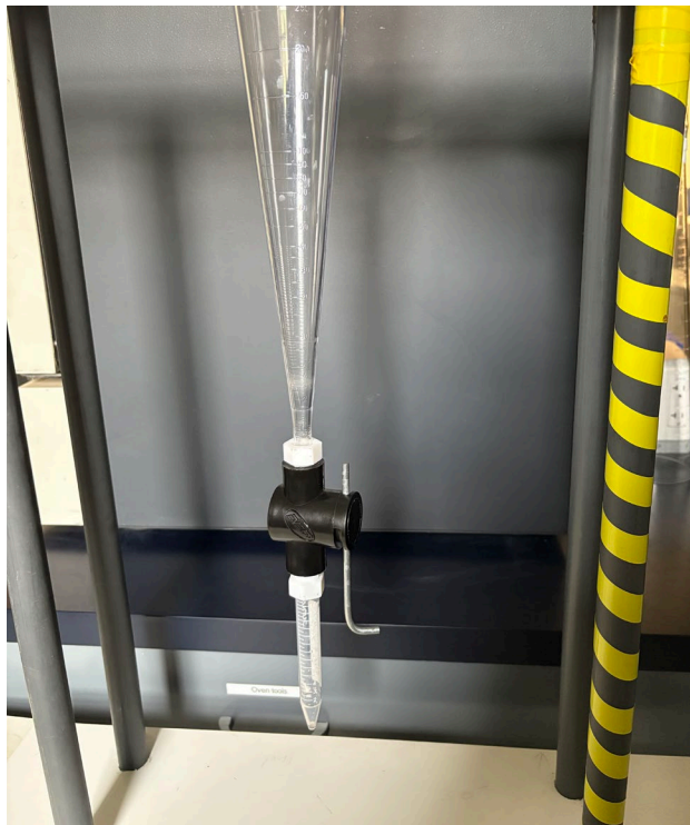
Figure 3. —An Imhoff settling cone with 3D printed coupler attached to a 15 mL collection tube.
