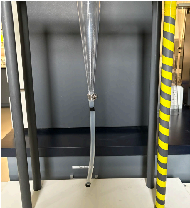
Figure 2. —An Imhoff settling cone with 3/8-inch ID tubing attached, marked to denote where to add clamps to collect 15 mL volume from settled sample.
