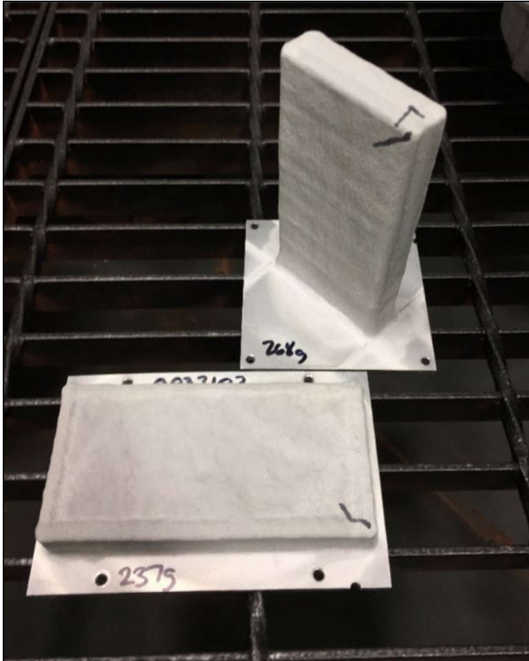
Figure 3.—Cold spray-printed 6061 aluminum blocks printed in the Z- and XY-directions [52].
