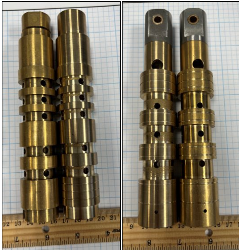
Figure 4.—Machined aluminum bronze additively manufactured parts compared to original parts removed from service. Left: Gate limit valve (additively manufactured part on right). Right: Section control valve (additively manufactured part on left).
