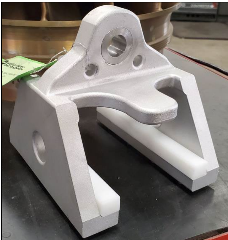
Figure 6.—Printed log boom anchor with stainless steel shackle insert and Delrin rails.
