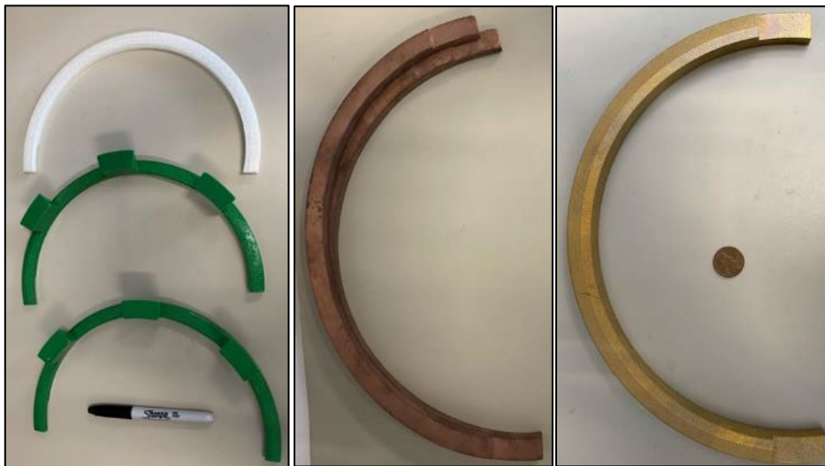
Figure 7.—Printed slinger ring PLA casting patterns (left), naval brass castings (center), and printed aluminum bronze slinger rings (right).
