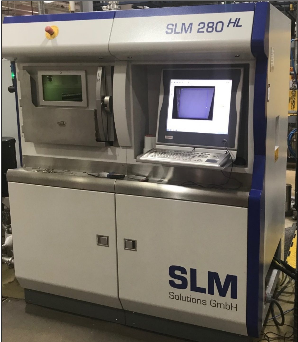
Figure 1.—SLM 280 HL machine used to build a 5- by 5-inch open cube with 316L stainless steel powder. Photograph courtesy of Concurrent Technologies.
