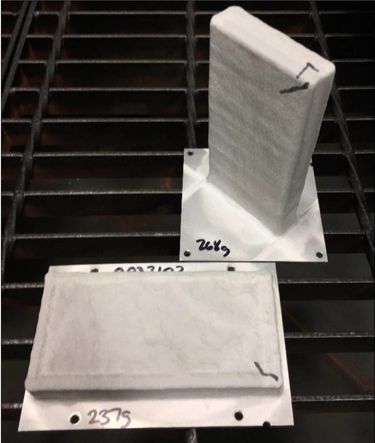
Figure 1.—Cold spray Al 6061 blocks printed in the Z (top) and XY (bottom) directions.
