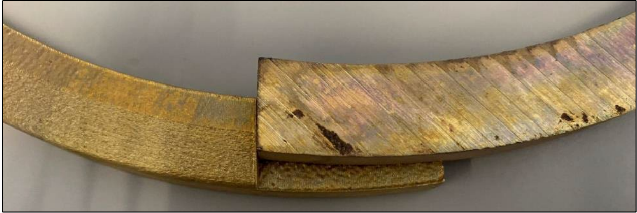
Figure 52.—Representative photograph of the joint between two direct-printed slinger ring halves. Warpage and dimensions being out of tolerance cause the halves to not meet correctly. The left side of the photograph shows the top (based on print orientation) of ring half A2527 and the right side shows the bottom of ring half A2240.
