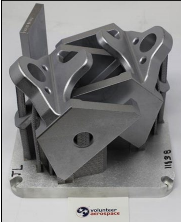
Figure 35.—Redesigned anchor parts and wall produced by additive manufacturing in as-printed state.
