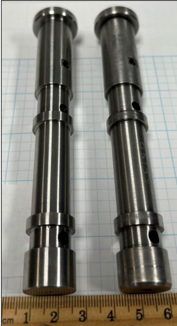
Figure 10.—Additively manufactured and machined pilot valve (Left) compared to original part (Right).
