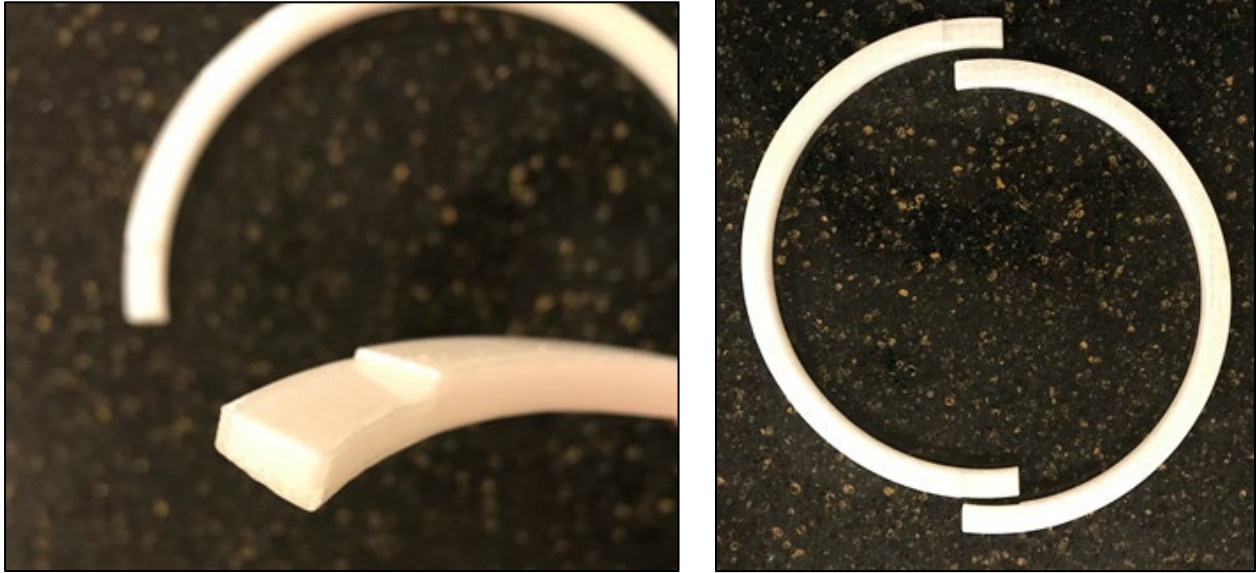
Figure 55.—Printed PLA ring halves to test the resolution for use as investment casting patterns.
