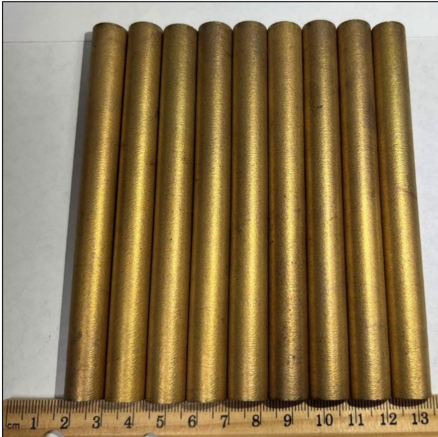
Figure 27.—As-printed aluminum bronze fatigue samples.
