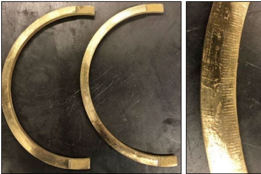
Figure 57.—Naval brass test castings prior to sand blasting to achieve final surface finish. Left: Two successful test castings. Right: Closeup view of surface texture on test casting.
