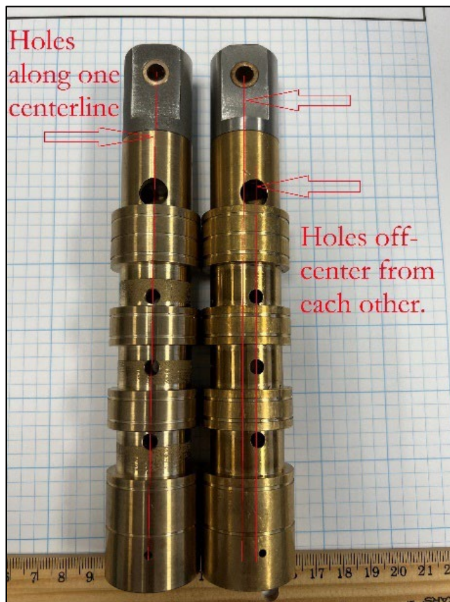
Figure 12.—Difference in hole alignment between printed pilot valve (left) and original (right).
