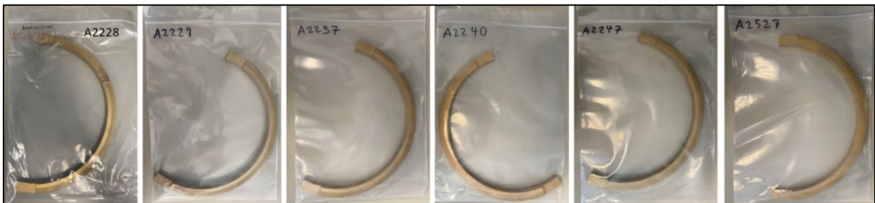
Figure 50.—Six slinger ring halves as-received from Elementum3D. The ring ID numbers are based on IDs that were inscribed on the parts by Elementum 3D.
