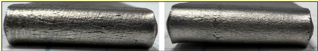
Figure 16.—Photographs of bend test samples after testing. Left: Sample 1 (parallel to Z-axis). Right: Sample 2 (perpendicular to Z-axis).
