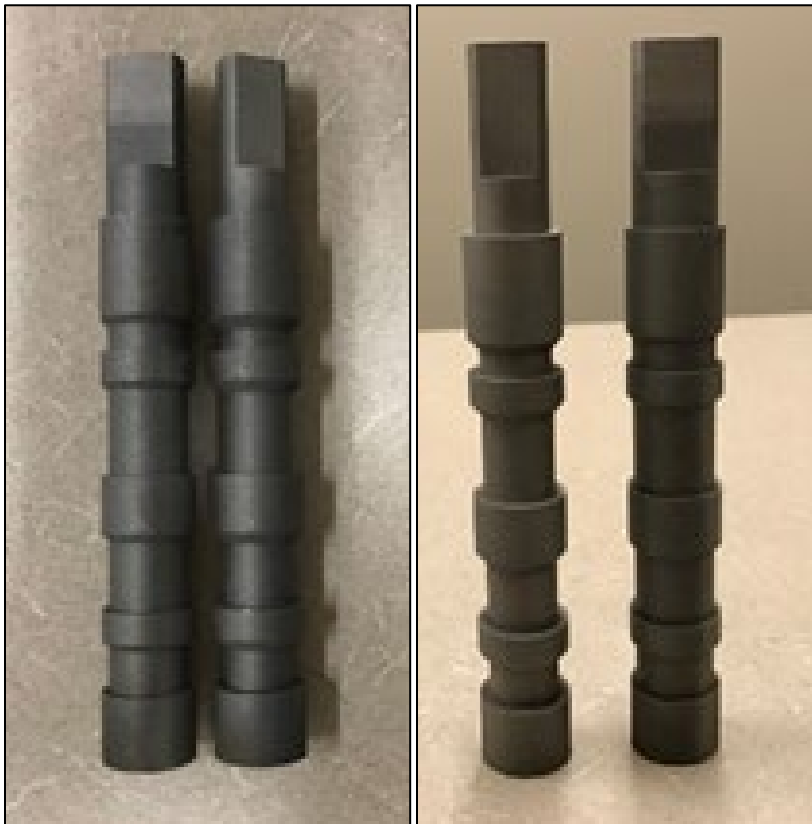
Figure 5.—3D-printed piston of gate limit valve. Left: Parts had material added to selected surfaces. Right: Parts had material added to all surfaces.
