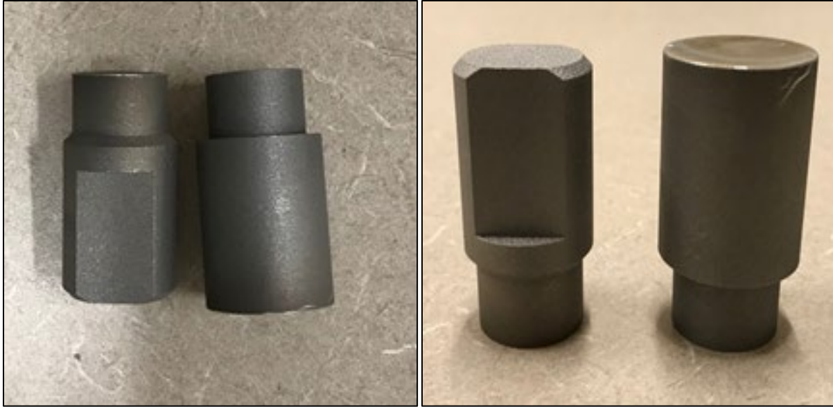
Figure 4.—3D-printed linking bars. Left: Parts had material added to selected surfaces. Right: Parts had material added to all surfaces.
