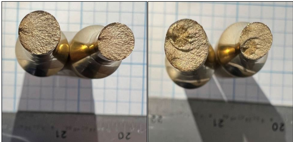
Figure 28.—Left: Fracture surfaces of specimen 12, run at 85% stress level. Right: Fracture surfaces of specimen 22, run at 95% stress level.
