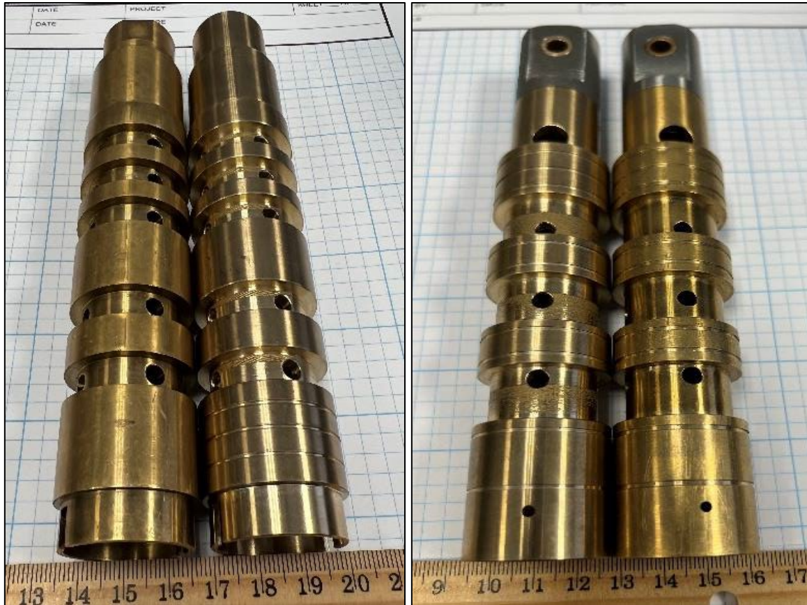
Figure 13.—Machined aluminum bronze additively manufactured parts compared to original parts removed from service. Left: Gate limit valve (additively manufactured part on right). Right: Section control valve (additively manufactured part on left).
