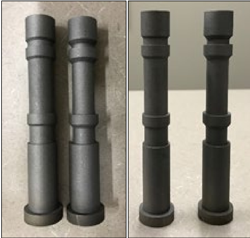
Figure 6.—3D-printed pin of pilot valve. Left: Parts had material added to selected surfaces. Right: Parts had material added to all surfaces.
