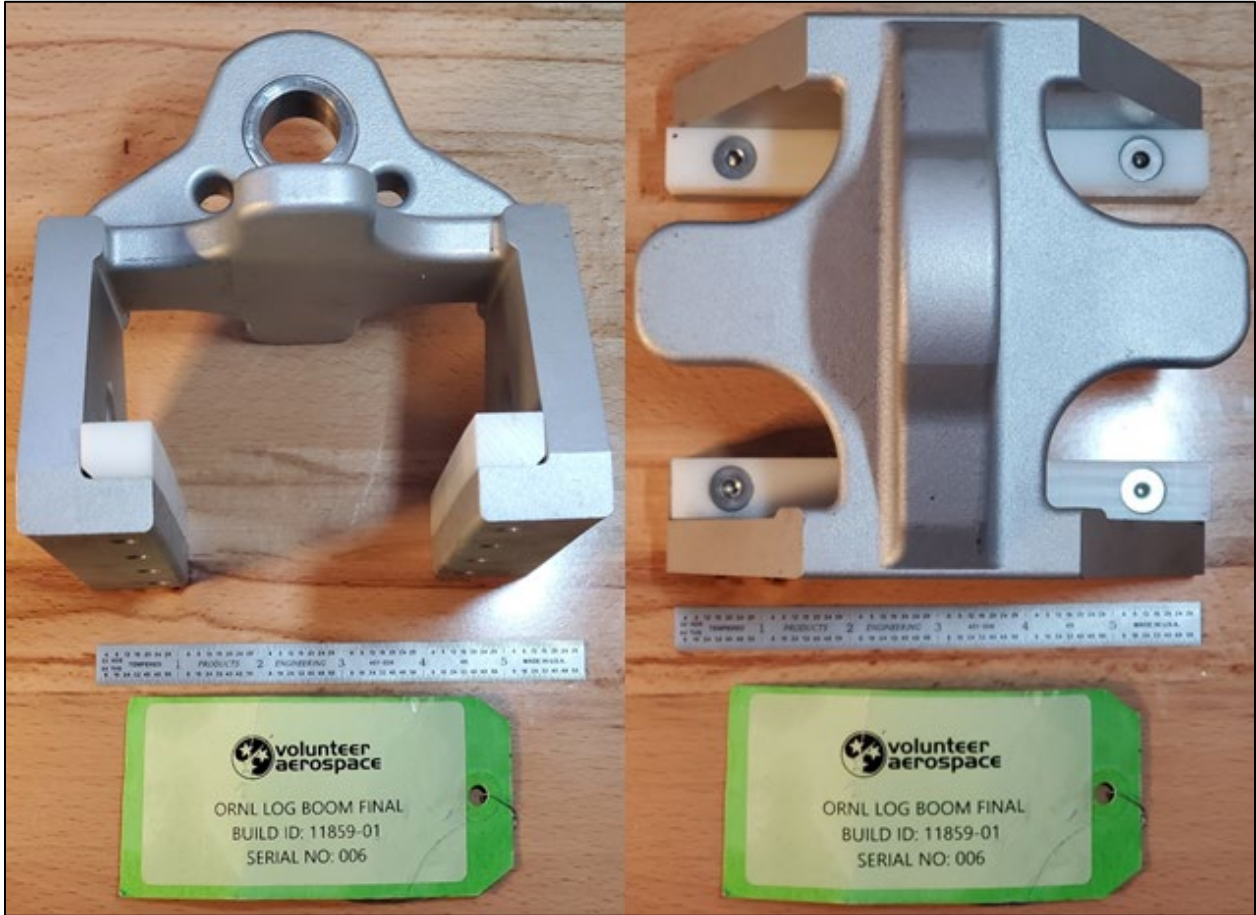
Figure 37.—Side and top view of the finished anchor blocks with the Delrin rails attached and the stainless steel insert pressed into the top shackle.
