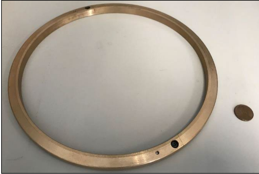
Figure 48.—Spare slinger ring received from Grand Coulee.
