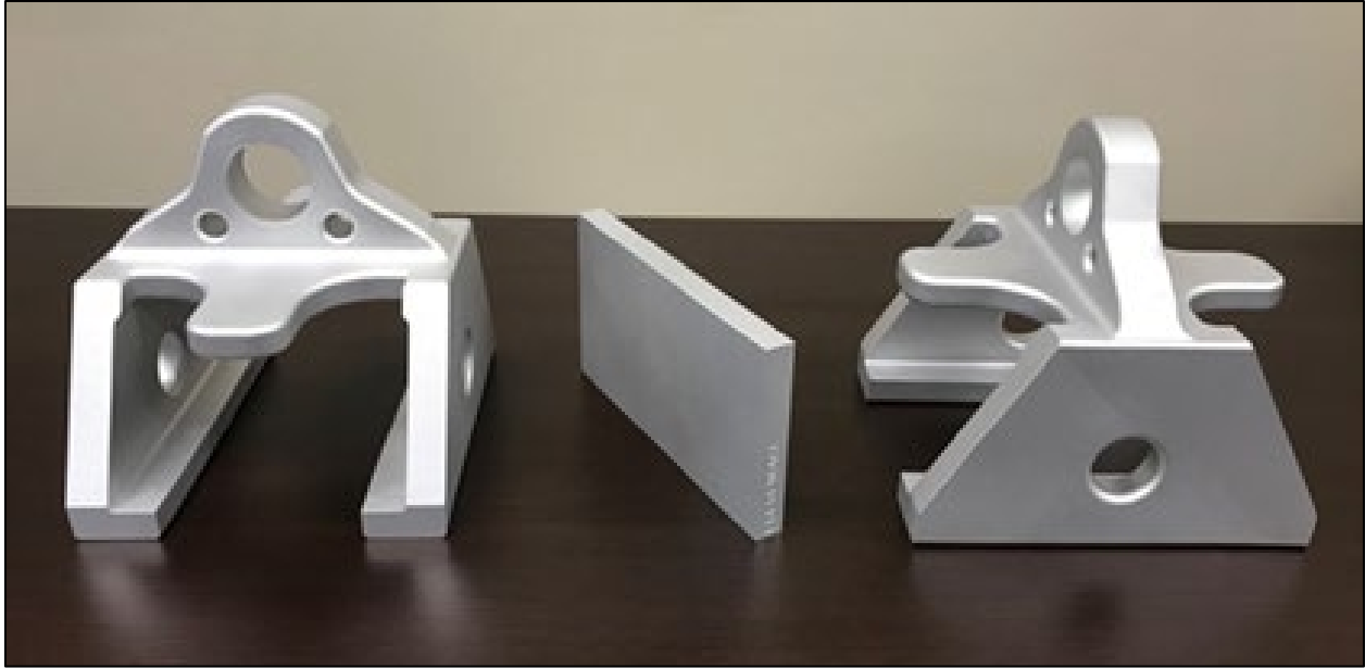
Figure 36.—Redesigned anchor parts and wall produced by additive manufacturing after post-processing.
