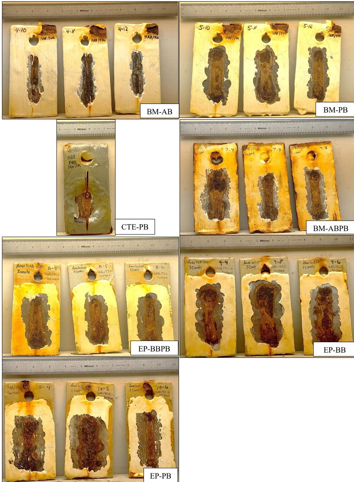
Figure 7.—Photos showing rust creep after 30 weeks of alternating exposure (HAR+FOG).
