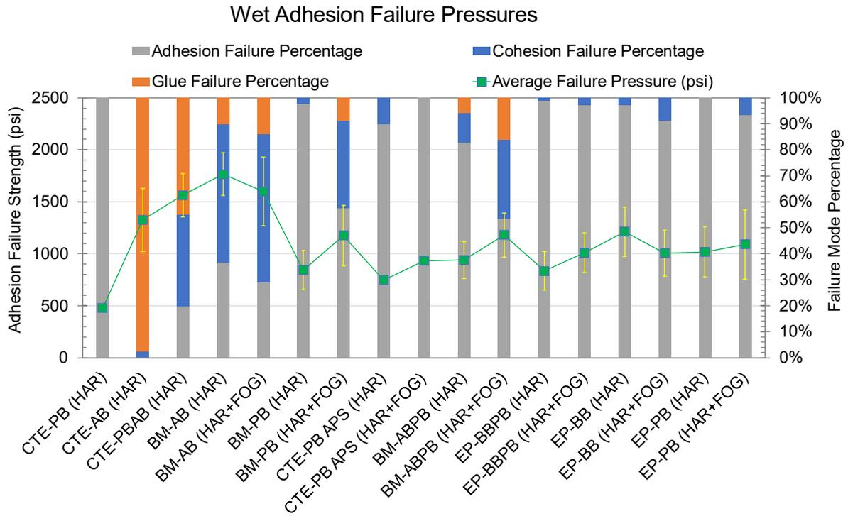
Figure 4.—Results of wet adhesion testing are plotted with the failure mode percentages for each material group.
