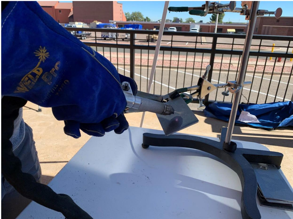
Figure 1.—Sample preparation using the PlasmaBlast™ system.
