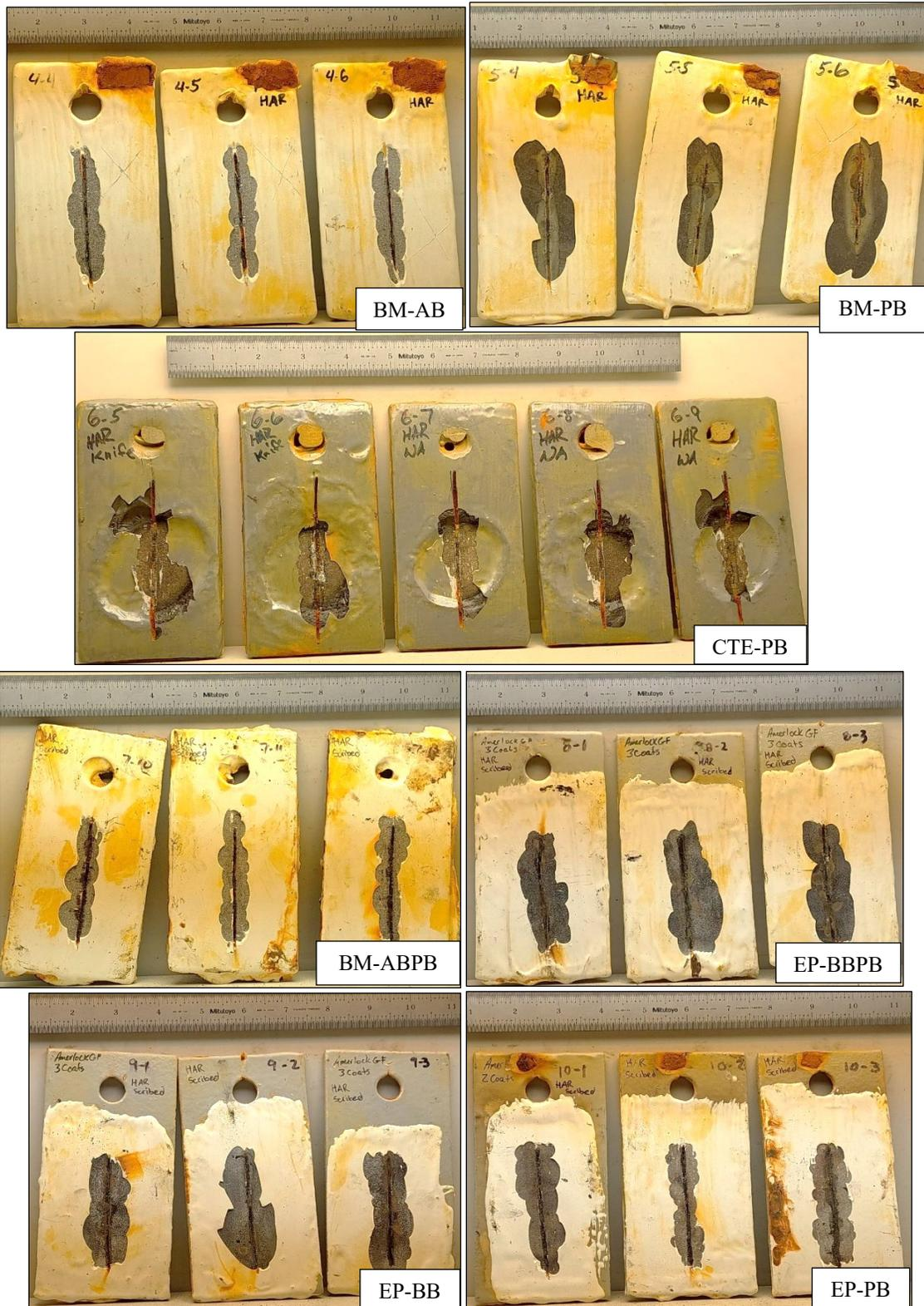
Figure 8.—Photos showing rust creep after 30 weeks of immersion exposure (HAR).
