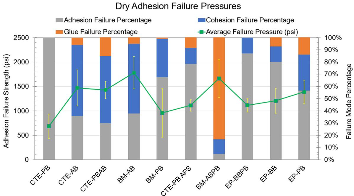
Figure 3.—Results of dry adhesion testing are plotted with the failure mode percentages for each material group.
