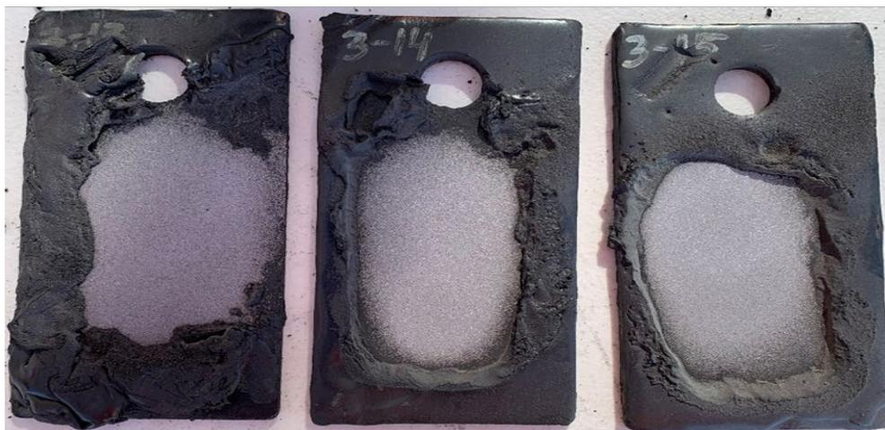
Figure 2.—Group 3 test panels shown after CTE removal with PlasmaBlast™ (PB) in the top image and with PB followed with dry abrasive blasting (AB) in the bottom image. The melted CTE along the perimeter of the blast area is not acceptable for spot repairs.
