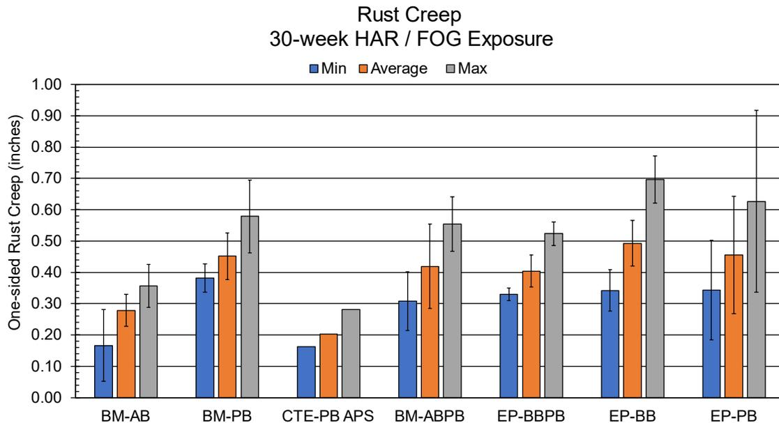
Figure 6.—Rust creep after 30 weeks of alternating exposure between HAR and FOG. Error bars represent plus or minus one standard deviation for values from a set of three or more test panels. Only one panel was evaluated for CTE-PB APS.
