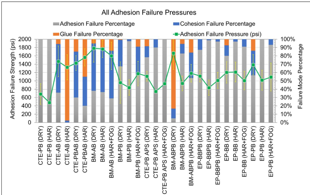
Figure 5.—Results of dry and wet adhesion testing are plotted with the failure mode percentages for each material group. Error bars represent plus or minus one standard deviation for values from a set of three or more test panels.
