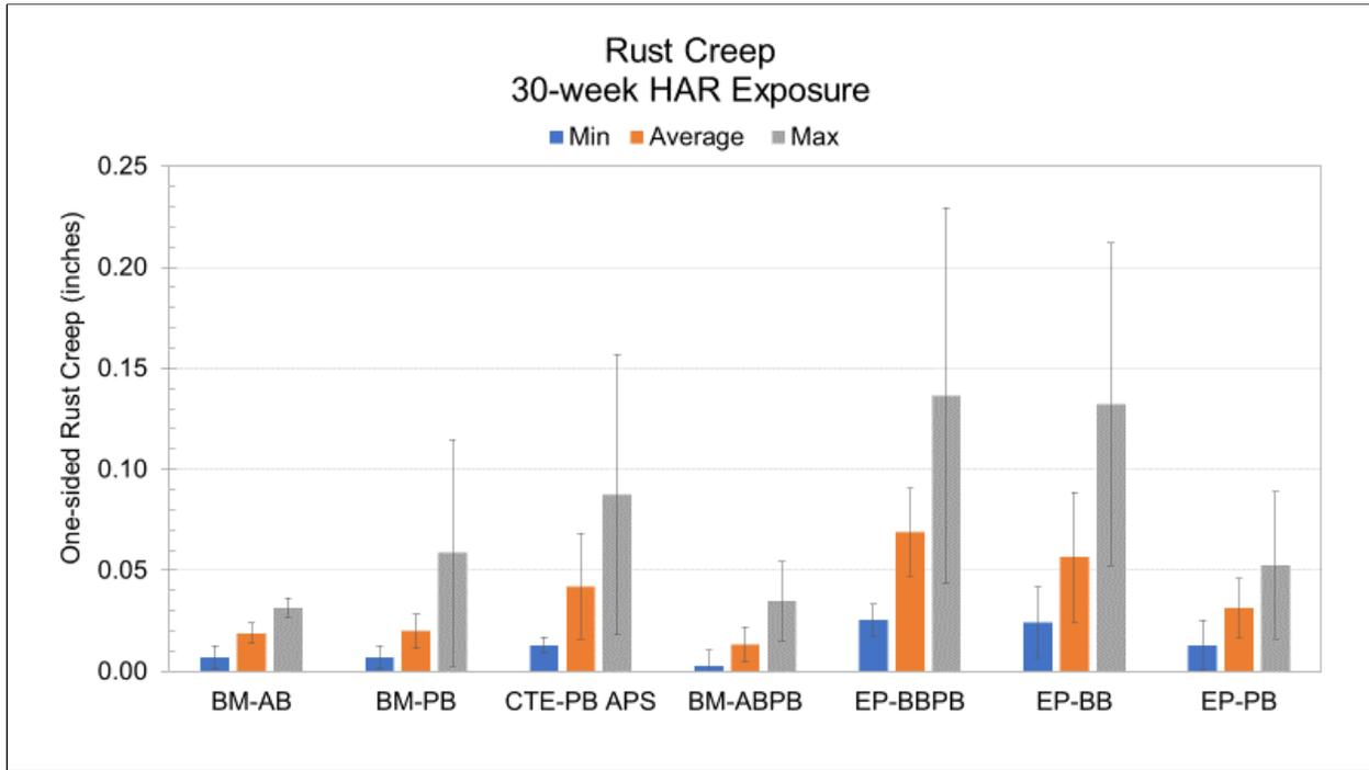
Figure 7.—Rust creep after 30 weeks of HAR exposure.
