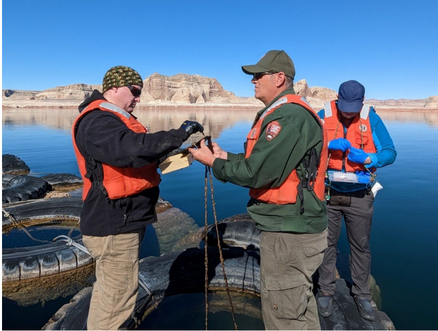
Figure 6. Collection of settled mussels and other biofouling species at the SLB site after Test 2.
