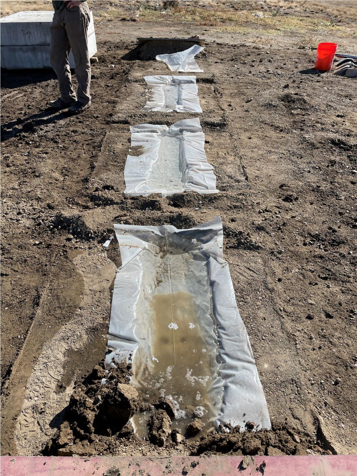
Figure 19.—Photo of water-filled visqueen films that were placed under each of the four concrete slabs.
