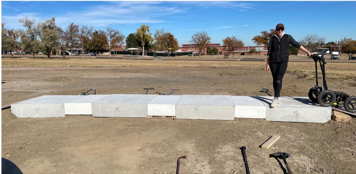
Figure 15.—Photo of field experiments showing each of the four concrete slabs. Slab 1 had no reinforcement (N), Slab 2 had a mesh reinforcement (M), Slab 3 had a single rebar mat (SM), and Slab 4 had a double rebar mat (DM).
