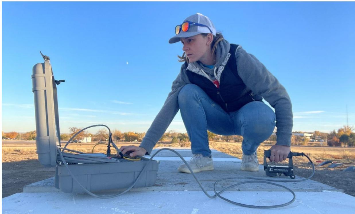
Figure 12.—Photo of Impact Echo data collection on the experimental slabs. The grey box (left) is the laptop and datalogger which attaches to the IE instrument (right).
