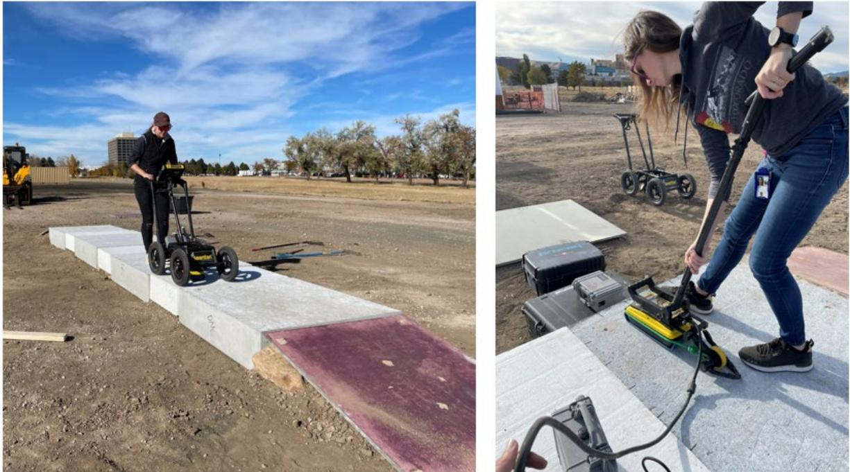
Figure 11.—Photos of GPR data collection at the Denver Federal Center using a (left) cart-based system and (right) handle attachment. Each system has a built-in odometer wheel to track distance surveyed.
