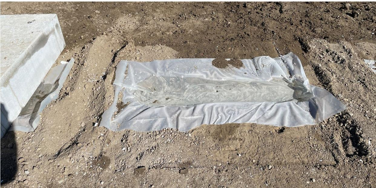
Figure 18.—Photo of longitudinal tunnel hand dug under the long axis of the experimental setup. A layer of visqueen plastic film was used to prevent the added water from draining during surveys.
