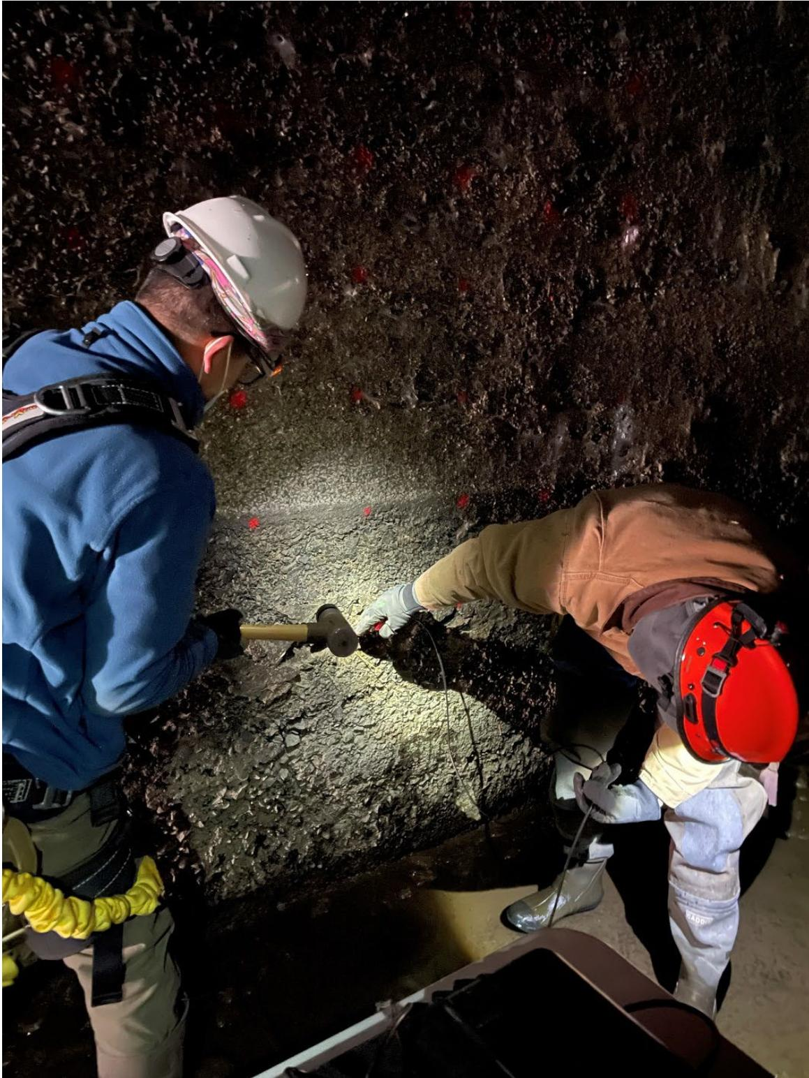
Figure 36.—Photo of Reclamation personnel performing one of the slab-impulse response surveys within A Canal.
