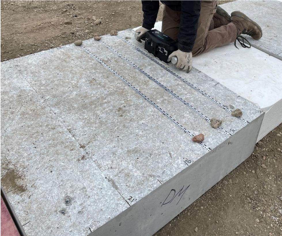
Figure 17.—Photo of concrete blocks with survey grid marked along the edges to indicate total distance along the survey grid. This photo shows block 4 marked from  $x=18$  to 22ft.
