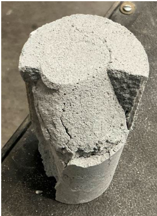
Photograph 13.—Strength specimen 32-20 after testing with failure occurring at “lift lines”.
