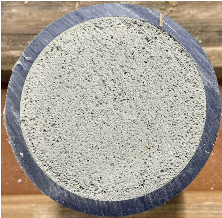
Photograph 19.—Section of 8-6.5 specimen with greater voids indicating lower density, higher porosity.
