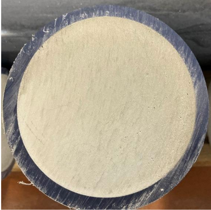
Photograph 8.—Section of 32-0.5 specimen with little to no voids visible indicating high density, low porosity.
