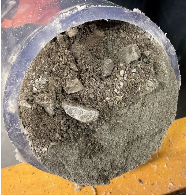
Photograph 27.—PLDCC specimen from 8-foot horizontal-debris, with unbound coarse and fine aggregate debris material.
