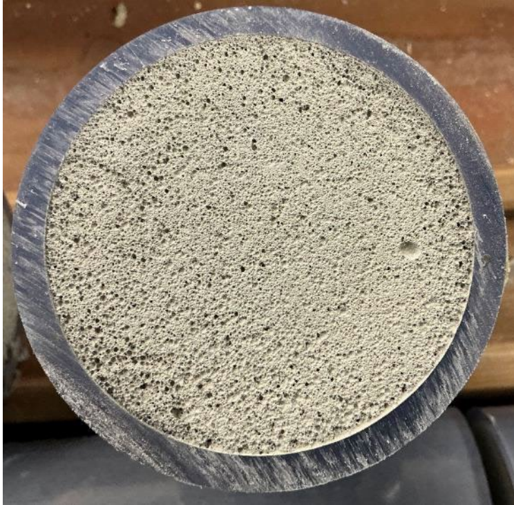
Photograph 16.—Section of 24-18.5 specimen with voids visible indicating low density, high porosity.
