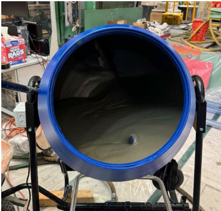
Photograph 2.—Fully mixed PLDCC in drum mixer.
