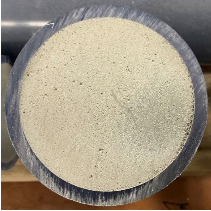
Photograph 15.—Section of 24-0.5 specimen with little to no voids visible indicating high density, low porosity.
