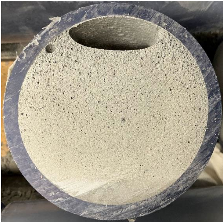
Photograph 22.—PLDCC specimen from 8-foot horizontal-empty, with air void and lower density at top, and higher density at bottom.
