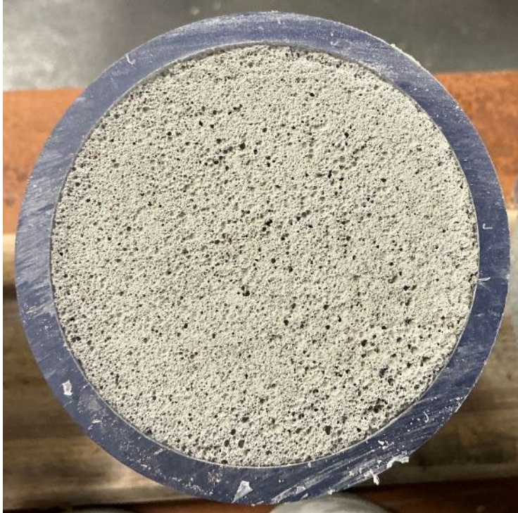
Photograph 9.—Section of 32-30 specimen with voids visible indicating low density, high porosity.
