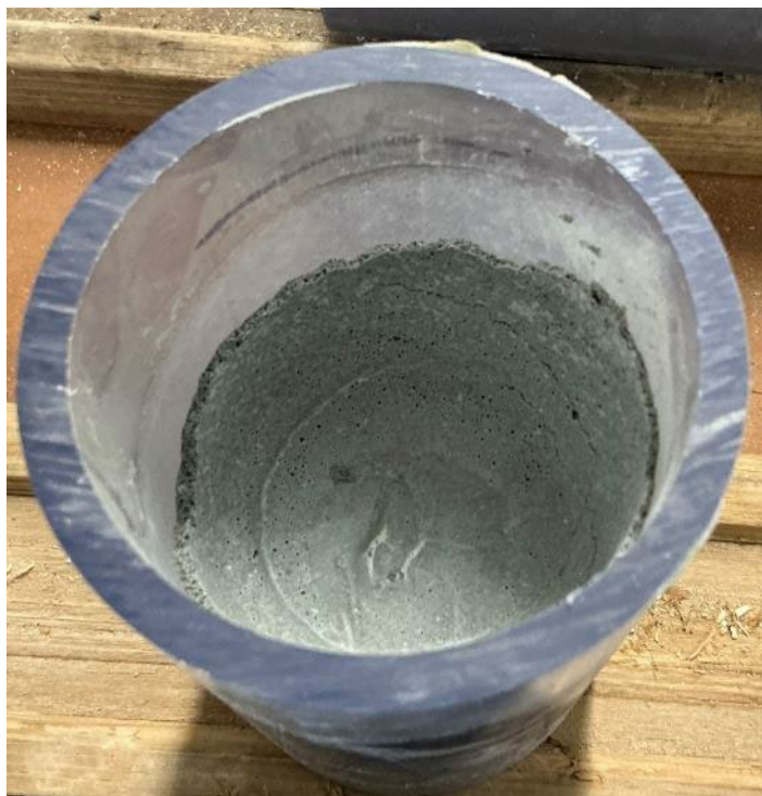
Photograph 20.—Collapsed upper extents of 8-foot set-up, approximate elevation 7ft.
