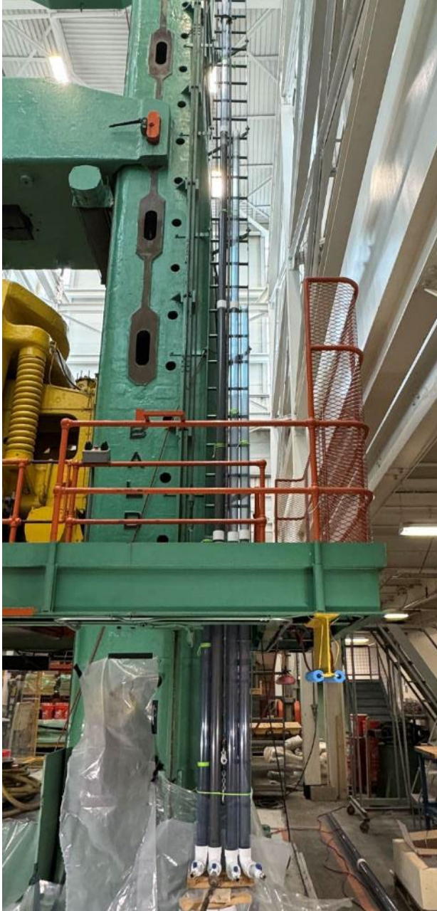
Photograph 4.—PLDCC test set-ups with vertical pipes attached to permanent ladder.
