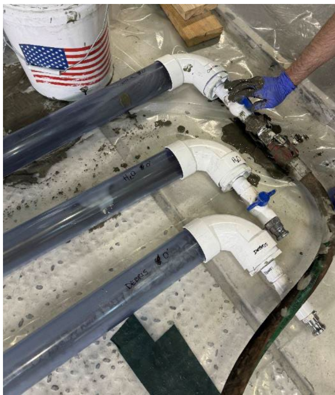
Photograph 6.—PLDCC pumping into horizontal 8-foot set-ups.
