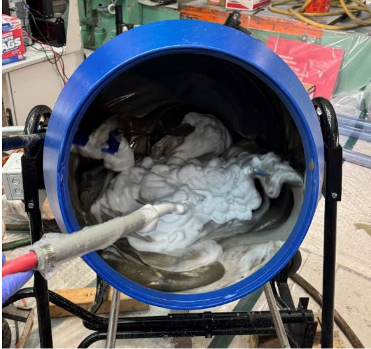
Photograph 1.—Addition of foam to cementitious grout in mixing drum.
