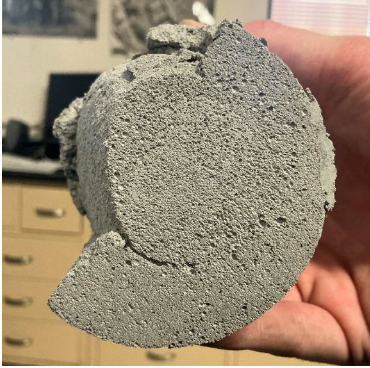
Photograph 12.—Strength specimen 32-20 after testing with failure occurring at “lift lines”.
