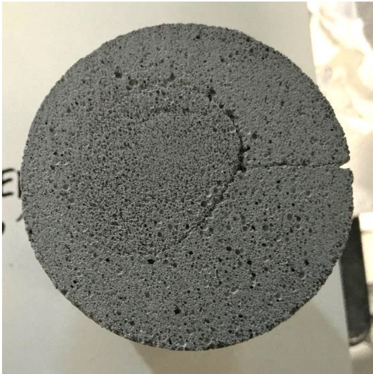
Photograph 11.—Strength specimen 32-20 indicating non-homogenous section and "lift lines".
