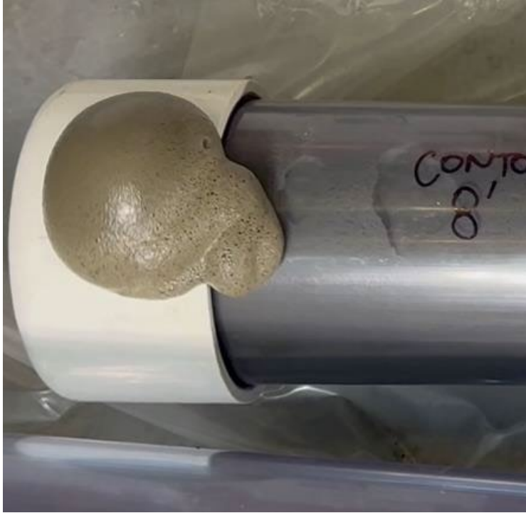
Photograph 21.—PLDCC discharging from vent hole of 8-foot horizontal-empty sample.
