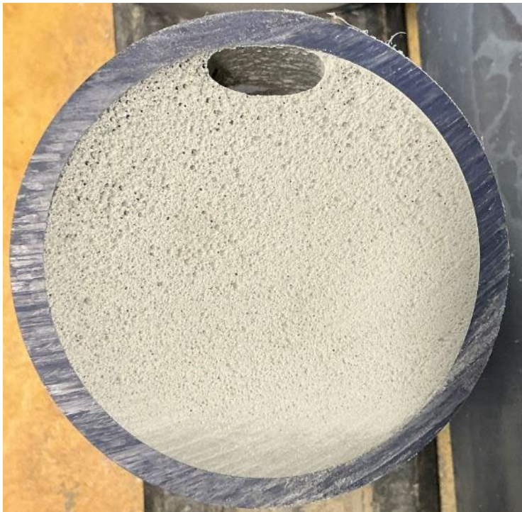
Photograph 25.—PLDCC specimen from 8-foot horizontal-water, with air void and lower density at top, and higher density at bottom.
