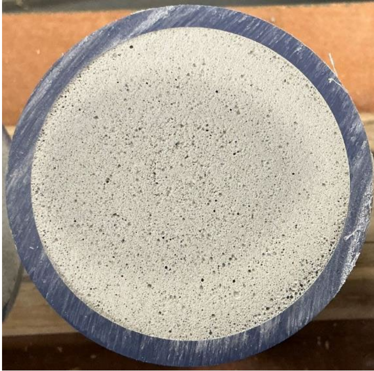
Photograph 18.—Section of 8-0.5 specimen with fewer voids indicating higher density, lower porosity.
