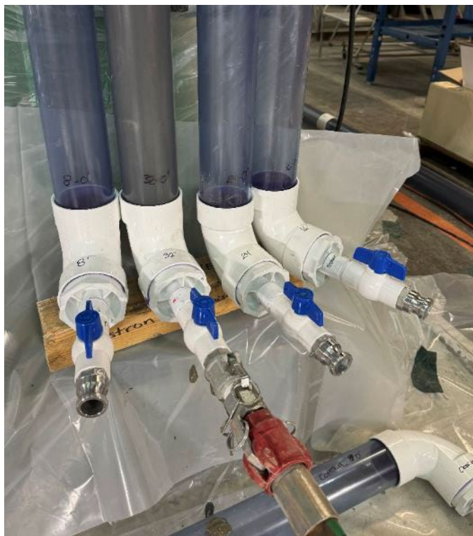
Photograph 5.—PLDCC pumping into vertical 32-foot set-up.
