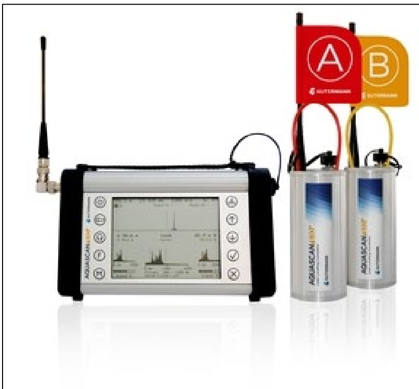
Figure 7.—Example photo of a wireless mobile correlator system with two sensors (“A” and “B”) and a system console that performs signal processing, cross-correlation, and leak locating calculations in real-time. In this example, the two sensors are mounted directly onto the pipeline or other metallic access points with built-in neodymium magnets integrated into the bottom of the sensor housing. Figure modified from (Gutermann, 2025).
