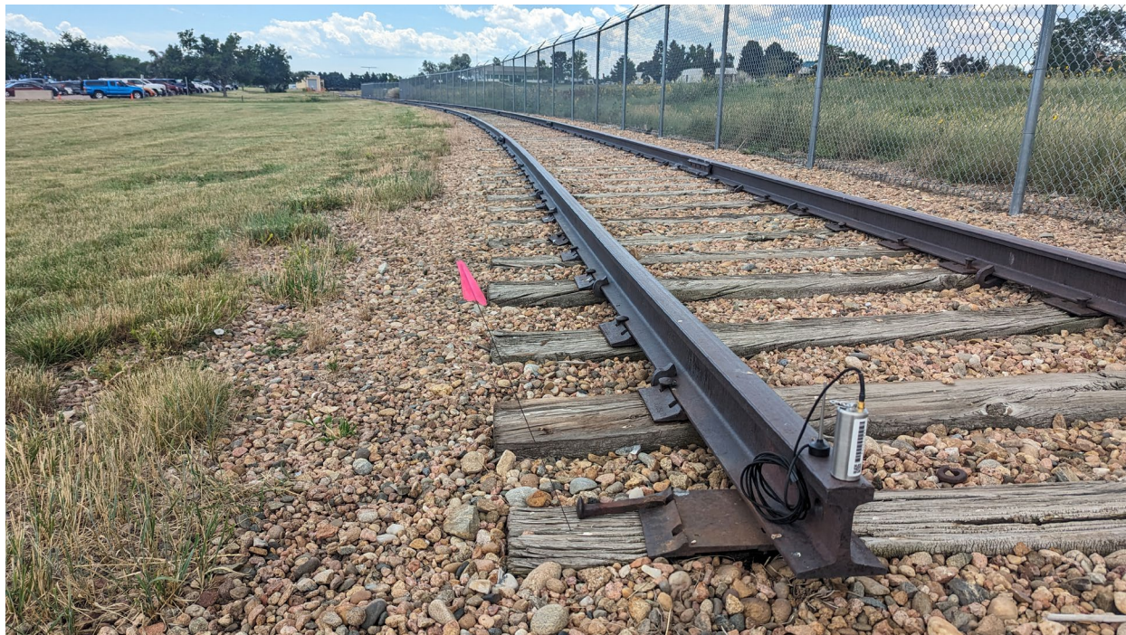
Figure 25.—Photo showing one of the Nb-IoT loggers (“Logger #1”) deployed at the northern end of the train track testing segment. As designed, each logger is firmly attached to the track using the neodymium magnet integrated into its base.
