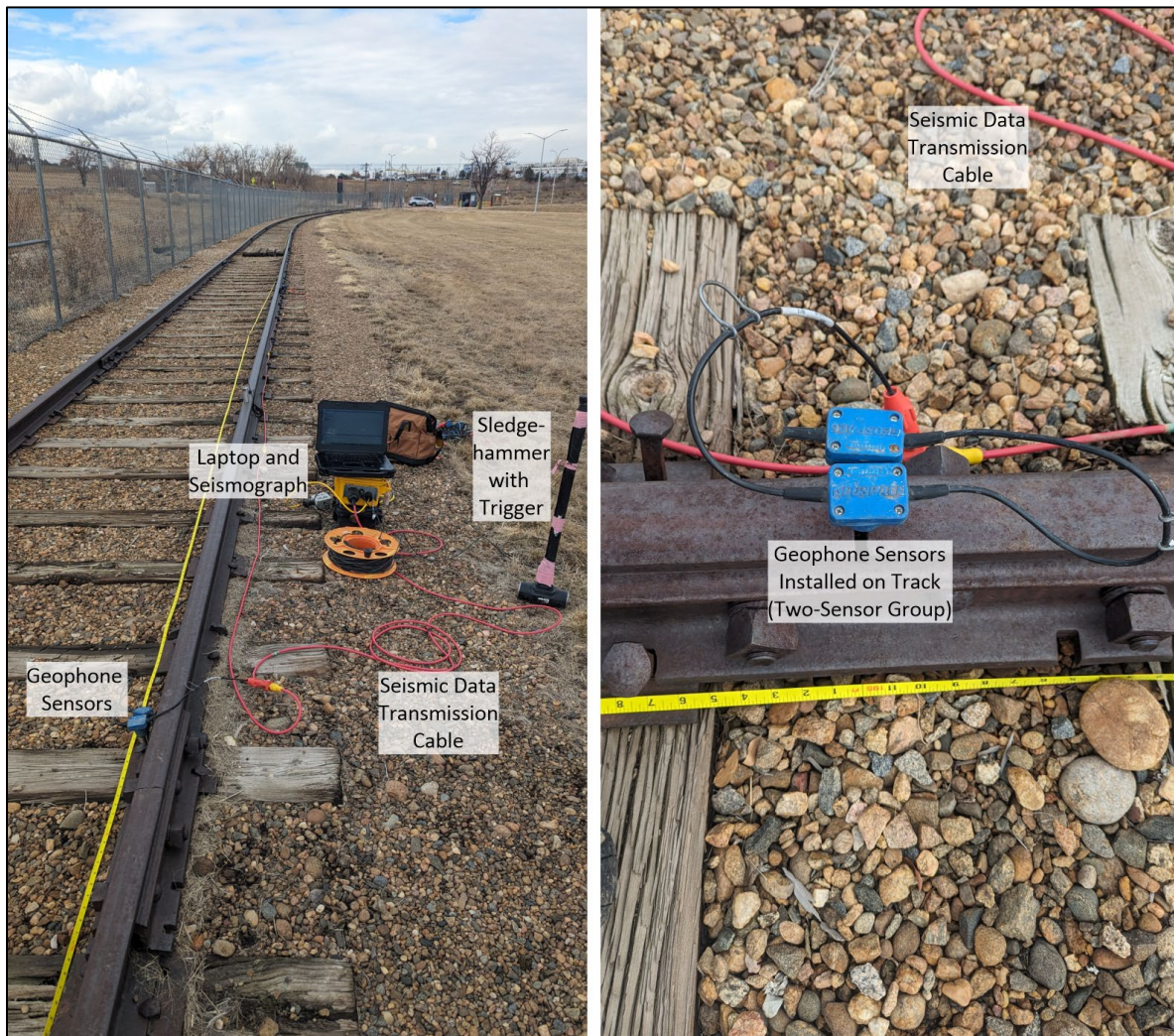
Figure 27.—Photos showing geophone sensors and seismic surveying equipment used to perform hammer tap tests for wave velocity analysis along the train track segment.
