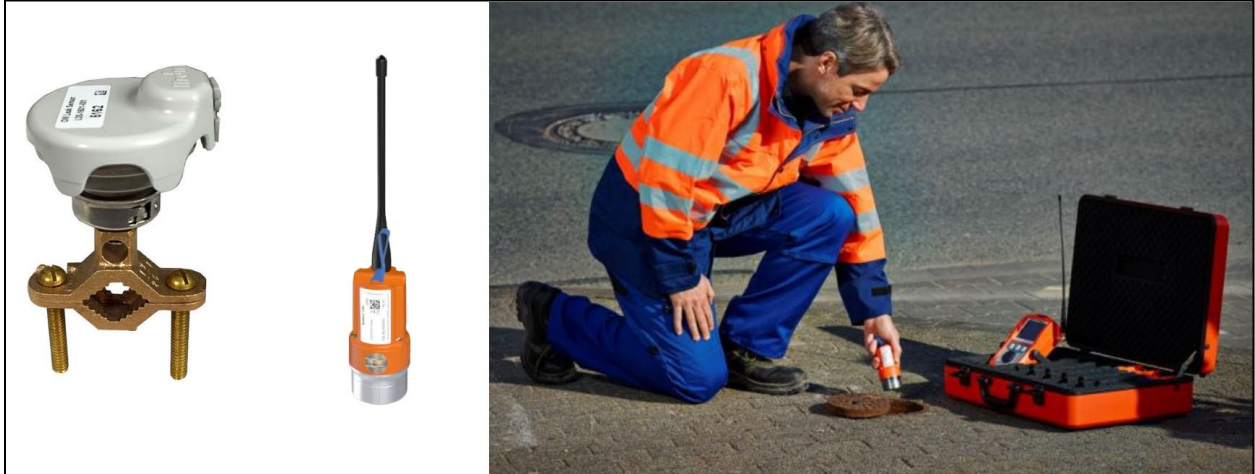
Figure 6.—Photos showing difference variations of AE noise loggers (left and center images), and a photo of a noise logger being deployed in the field with a wireless radio data harvest console (right). Figure modified from (Dalaeli, J., and Lunsford, J., 2023; Sewerin, 2025).
