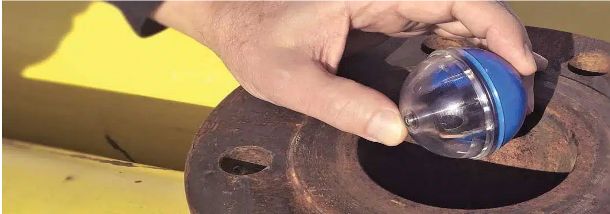
Figure 10.—Photo showing one of three variants of the in-line IGNU Inc. Pipers™ sensor system, approximately the size of a baseball. These devices are neutrally buoyant and are offered in three different sizes (1.50, 2.3. and 2.8 inches in diameter) to adapt to several internal diameters and access points from 2 in. and greater. This specific variant of the IGNU sensor only records movement, magnetic field strength, and thermal data. Figure taken from (Whitfield, S., 2025).
