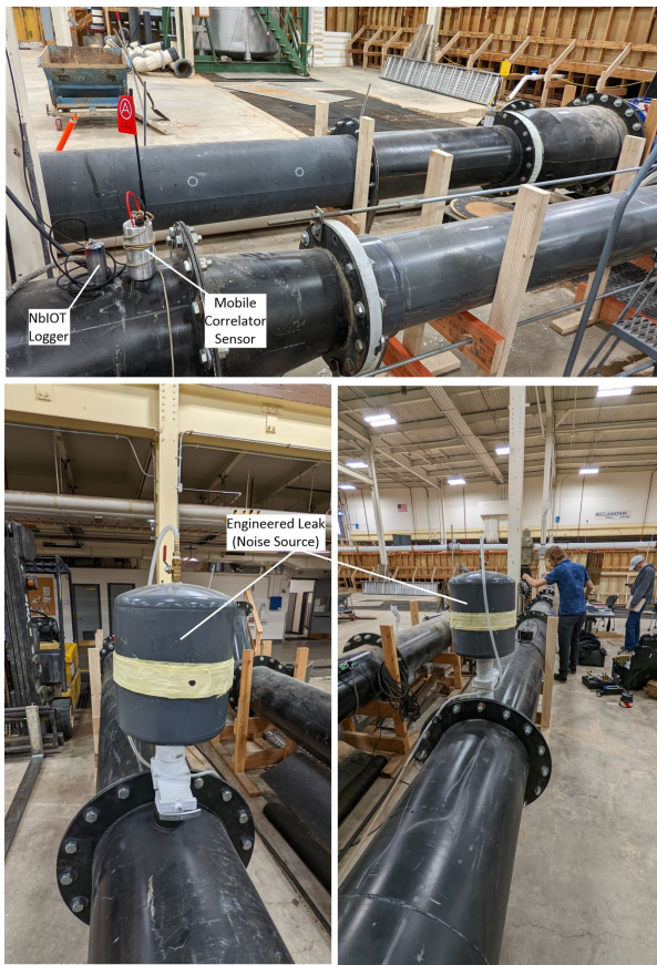
Figure 18.—Various photos taken during testing of Nb-IoT loggers in the Building 56 Hydraulics Laboratory.
