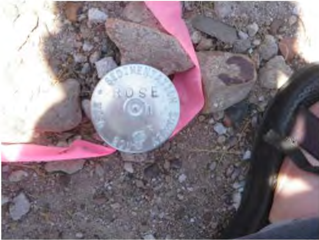
Figure 3 – “Rose 1” control point used as base for the 2013 hydrographic survey.
